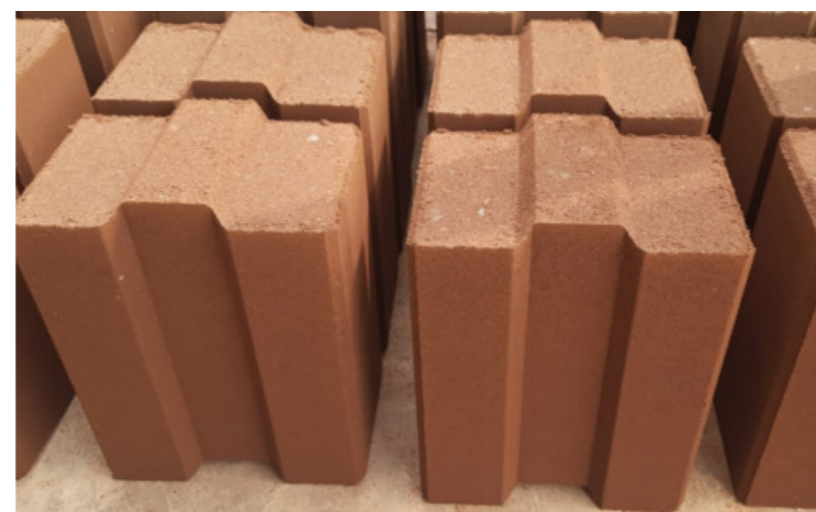
Red mud foamed concrete block. Photo ©
