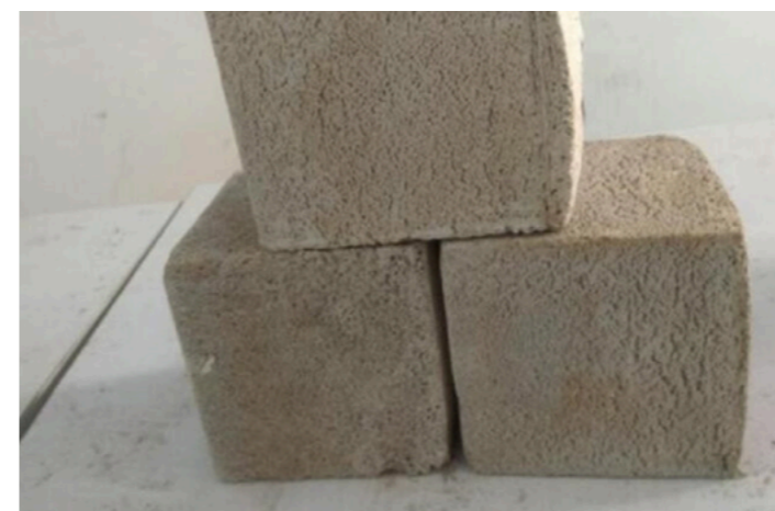
Iron-ore slag foamed concrete block. Photo ©
