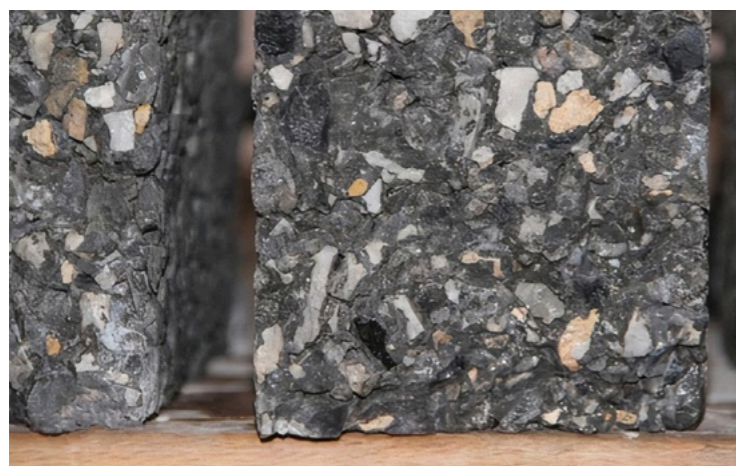
No-Fines Concrete with Steel Slag Samples. Photo © L.Korat et al., 2015. Image via ResearchGate.
